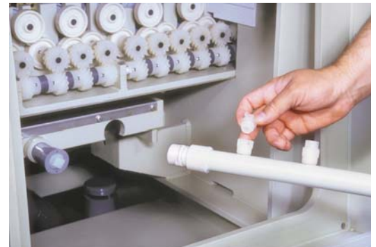
Quick-disconnect spray bars and nozzles
